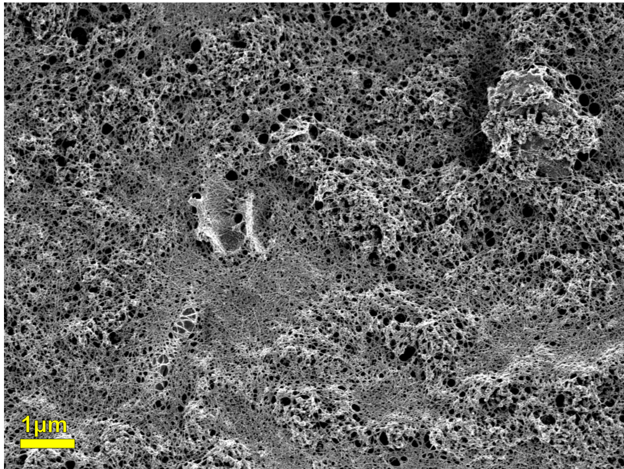
Figure S17: SEM image showing the draping of CNT particles on larger CB agglomerates after spraying onto filter paper.
