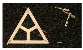
Fig. 4: A photograph of a complete ABS frame. Copper pads and lead wires can be seen at each of the triangle tips. Slightly visible is a Y-shaped frame stiffener adhered to the center cross members of the frame. Not visible are 50  $\mu$ m layers of VHB transfer tape affixed to the underside of the frame and between the frame stiffener and the frame.
