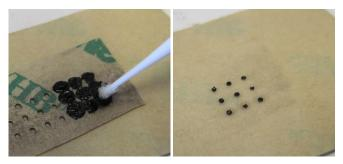
Fig. 5: The photographs on the left and right show the application of carbon grease through the polycoated paper mask onto the unstretched VHB film and the resulting alignment grid, respectively. The VHB film appears tan in these photographs because its paper liner is still attached.
