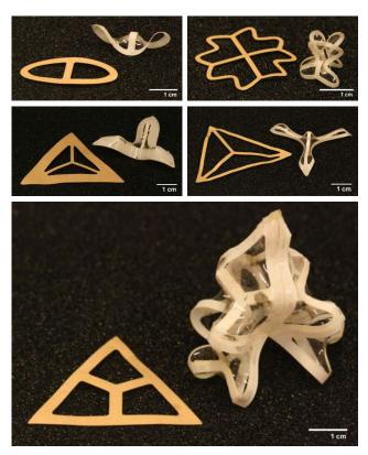
Fig. 1: Various inextensible, pliant planar frames adhered to 500% isotropically stretched elastomer films. The films are F9473PC VHB transfer tape from 3M and the frames are cut from 76.2  $\mu$ m thick ABS sheets. The object on the left of each 3D structure represents the original planar conformation of the frame. The bottommost object contains six of the triangular frames linked together along their edges.
