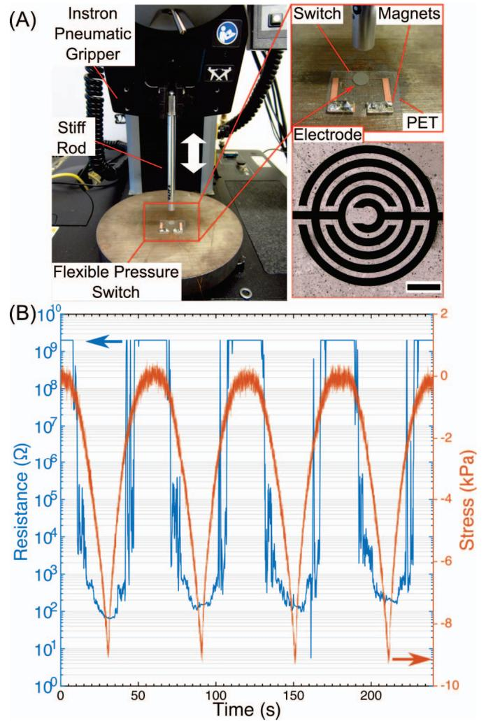
Fig. 3. Response of flexible pressure switch to normal pressure. (A) Experimental setup. Insets show close-up of test sample (top) and circular interdigitated electrode geometry (bottom, scale bar 1 mm). (B) Graph of in-plane resistance (i.e. resistance between the interdigitated electrodes, left y-axis, shown in blue) and normal pressure (right y-axis, shown in red) against time.
