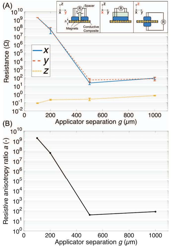
Fig. 2. Characterization of resistance of fabricated composite samples. (A) In-plane ( $x$  and  $y$ ) and through-thickness ( $z$ ) resistances as a function of applicator separation  $g$  (average of four measurements, error bars are  $\pm$  one standard deviation). Inset, schematic depiction of the experimental setup. (B) Ratio of the mean of the average in-plane resistances to through-thickness resistance,  $a$ , against applicator separation  $g$ .
